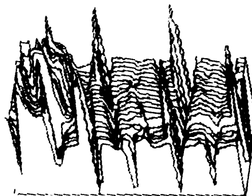
Figure 1 — A photothermal scan of a 6061 aluminum sample showing a series of subsurface cracks extending beyond the visible tip of a surface crack with a width of approximately 5 \mu\text{m} .
