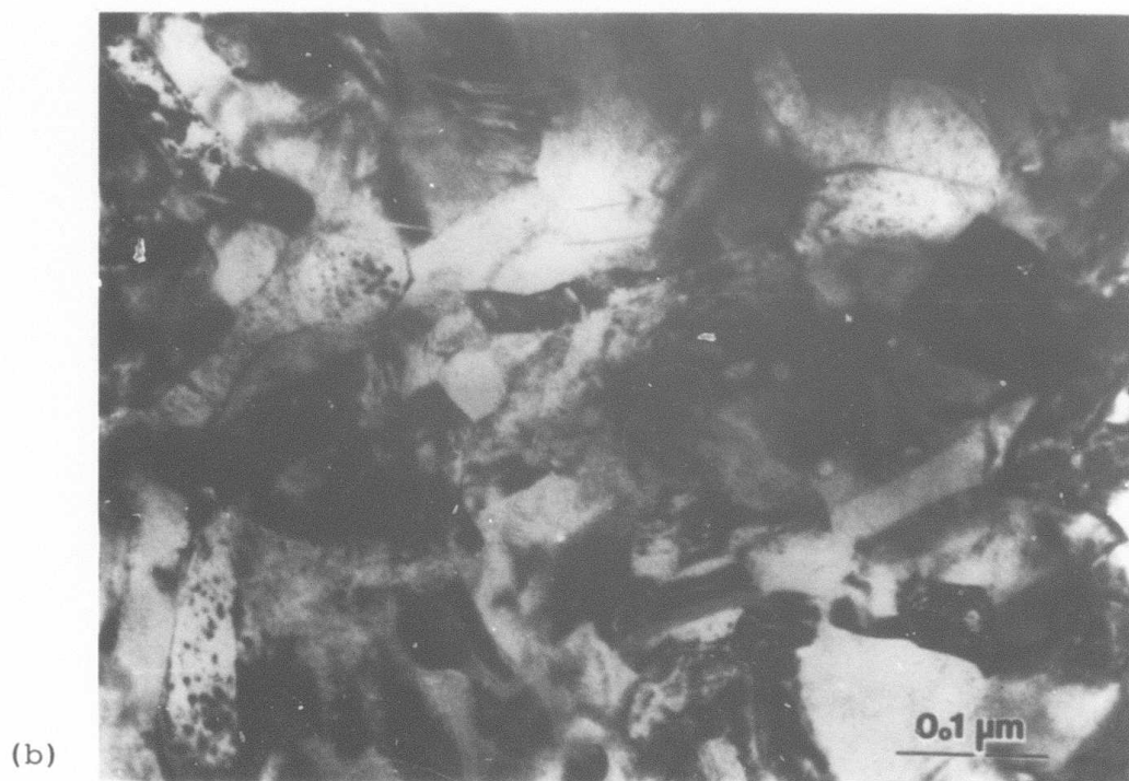
Figure 6: TEM micrographs of the top region of the ribbon. Melt-spun Co-34wt%Sn eutectic alloy.
