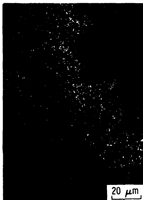
Fig. 7. (a) Scanning electron micrograph and (b) an EDAX W-map of the area near a laser burn on WC/C. Note the liquid matrix phase, the attack on the side and end of one carbon fiber, and the growth of carbon on the end of a cooler nearby fiber.
