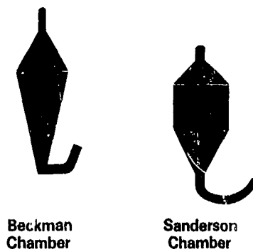
Fig. 3. Differences in chamber configurations for standard Beckman chamber and Sanderson chamber. Both chambers have significant differences that favor one chamber over the other in terms of cell collection or cell fractionation.
