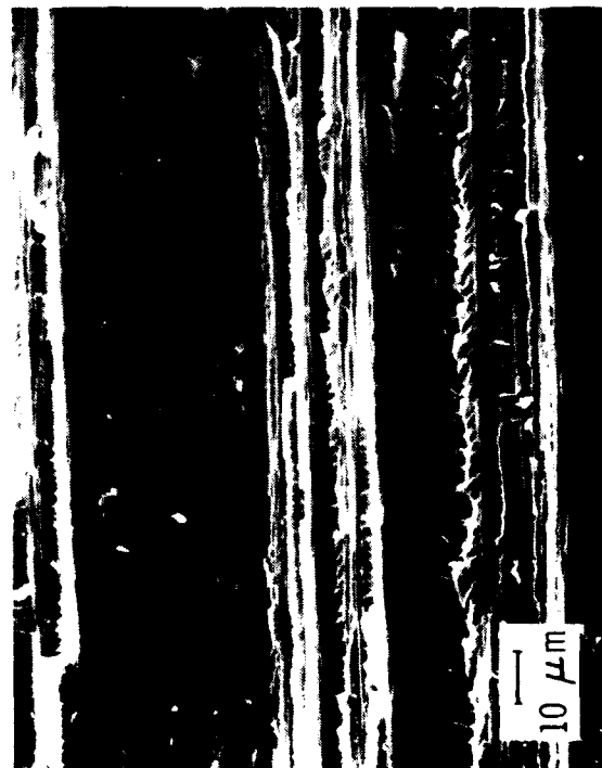
Figure 9. \beta = 45 deg, K_1/K_{II} = 1.0 , 7300/1034c
