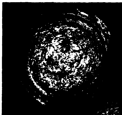
Fig. 20. Microstructure of a Sound Mesophase Rod Produced by Extrusion and Drawing
