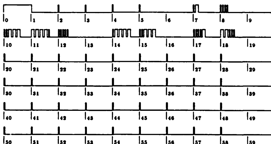
Figure 3.1. Time code format used to amplitude modulate the 10 KHz pilot tone for each minute. The minute begins with a 1040 ms pulse, and most seconds are marked by a 40 ms pulse, but the ninth of every ten seconds is omitted to facilitate counting tens of seconds. The two-character station ID is encoded during seconds 7-8, the day code during seconds 10-12, the hour during seconds 14-15, and the minute during seconds 17-18, all in Morse code. Shown is station AH (Arrival Heights), day 295, hour 12, and minute 47.
