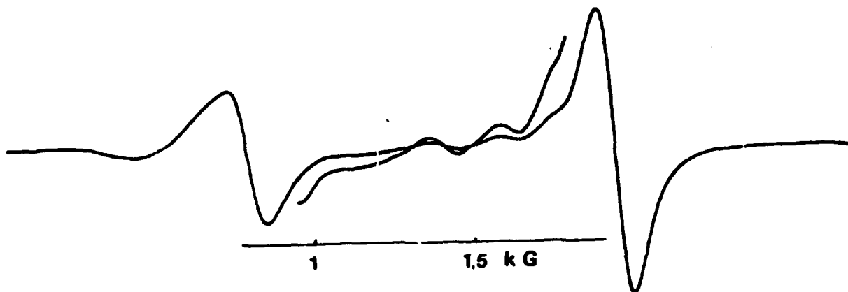
Fig. 3-5: Parallel resonance spectra for Film 84 After 250°C Anneal, f = 4.5 GHz
