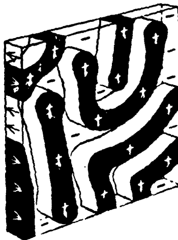
Fig. 1-1: Demagnetized State of Garnet Material with no Field Applied [1]
