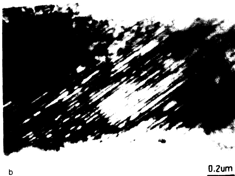
Figure 4.16 - TEM images of an Fe-32Ni specimen as cooled to -196^{\circ}\text{C} .
