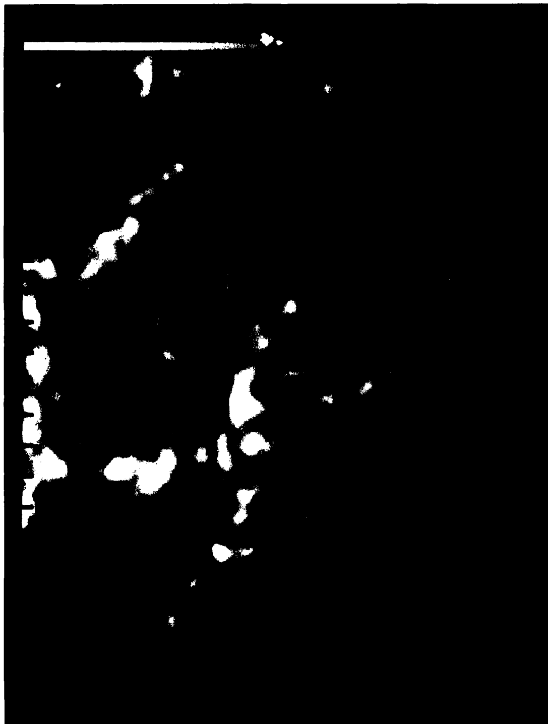
Magnetogram in Fe I 6302 made with the CID camera and video processor on the November, 1983, observing run. This frame was digitized from videotape. It shows the best seeing obtained in any run with the CID camera. Tick marks are 5 arcseconds.
