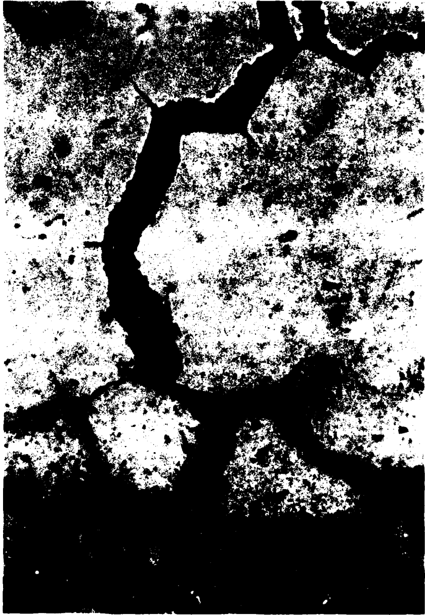
Figure 13. Grain Boundary Attack (500X) 6 .
