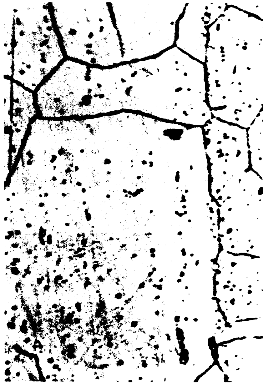
Figure 12. Formation of Precipitates by Carbide Accumulation.
