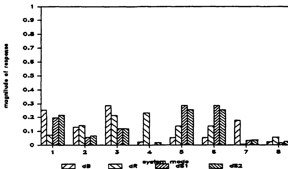
Figure 3.3 Controllability Analysis for the Linearized Roll Control Model.
