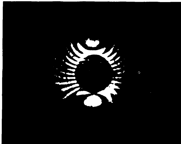
Figure 7. Interferogram between state #1 of test plate (relaxed), and state #2 (hanging weights) made in real time holographic system
