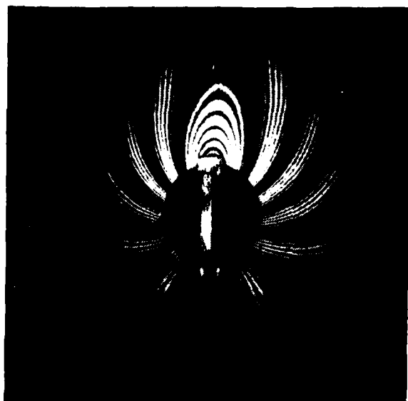
Figure 10. Four exposure moiré. The moiré is between two interferograms viewed from the hologram. The moiré compares to the low load interferogram shown in Figure 11.
