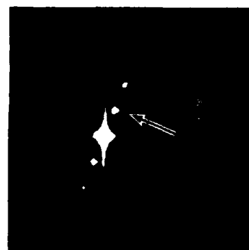
Figure 5c. Fourier spectrum of the reconstructed image of Figure 4c showing the delta functions in the (x-y) plane
