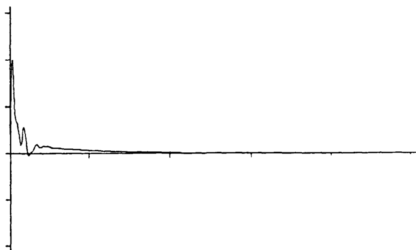
Fig. 11. Example 1 structure displacement/time K=9
