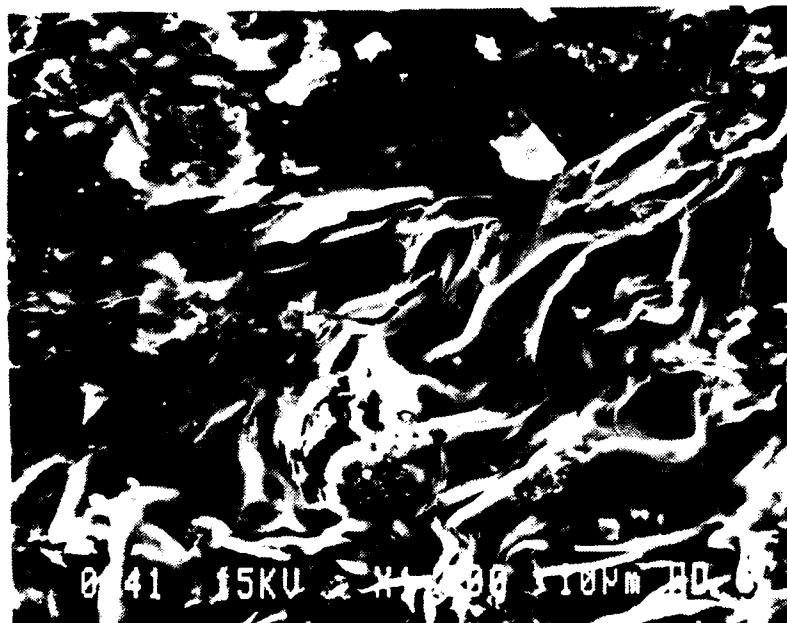
Fig. 34. SEM micrograph (1000x) of coal-tar pitch heat-treated to 2400°C for 30 minutes.
