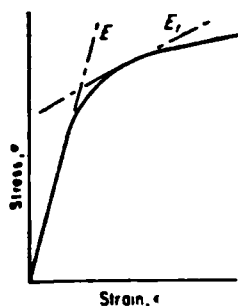
Fig. 1—Representation of tangent modulus.
