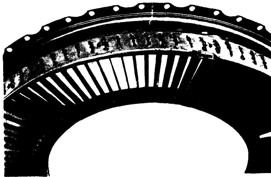
Figure 2. Coating failure and corrosion on the outer ends of the stator vanes where they pass through the shroud.
