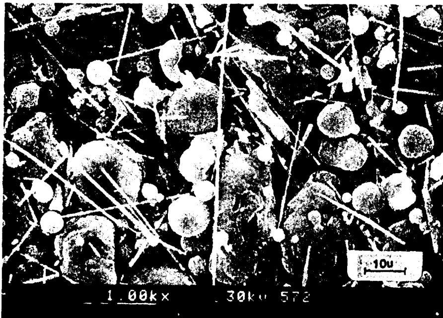
(b) Whiskers intimately mixed and randomly oriented around powder particles on a micro-scale
