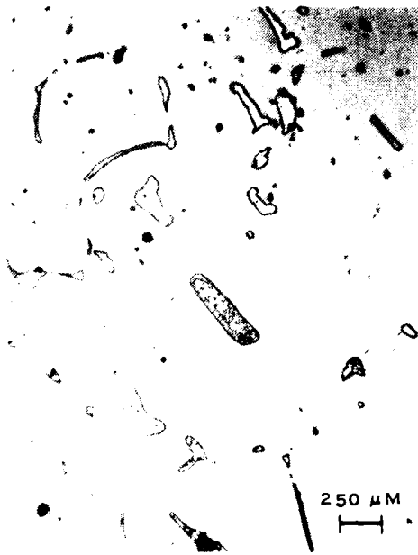
(A) GROWN UNDER LOW-THERMAL GRADIENT, < 50^{\circ}\text{C}/\text{CM} IN AIR
