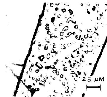
(B) MAGNIFIED SECOND PHASE EUTECTIC
