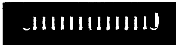
(b) Side view of chip carrier with solder bumps
