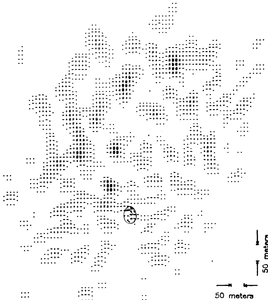
Figure 10a. Sample realization of an uncorrected irradiance distribution at the relay mirror. The shaded oval region denotes the size of the Airy disk of a diffraction-limited 1 meter transmitter; approximately 50 meter in extent, as indicated.
