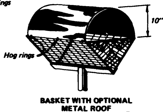
Figure 2. Design specifications for a rectangular basket nest structure for waterfowl (courtesy Harold A. Doty, U.S. Fish and Wildlife Service, Northern Prairie Wildlife Research Center)
