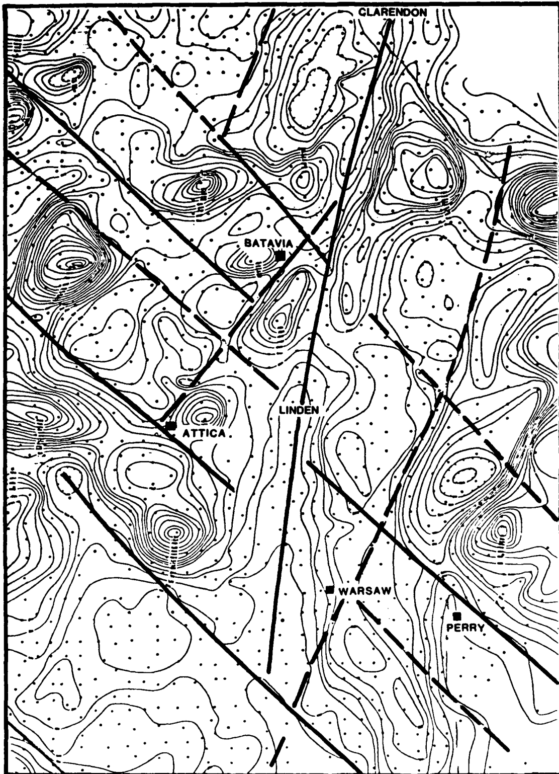
Figure 105. Magnetic map of Attica, New York and vicinity showing interpreted lineaments (modified from Thompson and Kujawski, 1975)
