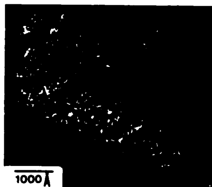
Fig. 2. Single crystal, as grown. Centered dark-field micrograph, bright regions are ordered microdomains.
