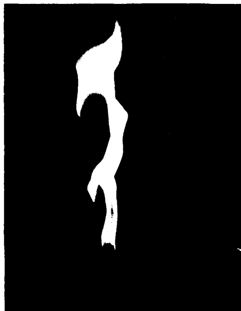
Fig. 4 R_p - 2000 turbulent diffusion flame; film exposure - 100 ms.
