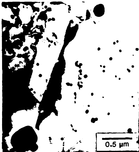
Fig. 1 - TEM micrograph of the as-processed microstructure of the RS Ti-2Er alloy.
