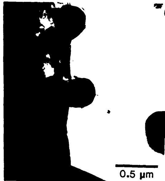
Fig. 2 - TEM micrograph of the RS Ti-2Er alloy following the beta grain growth anneal.
