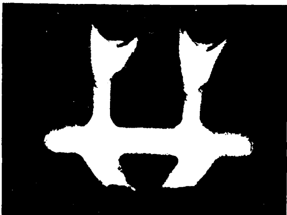
Figure 4-23. With no button present, the largest mass of metal is the reservoir bar.
