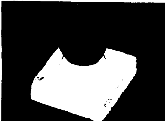
Figure 6-1. The oxide layer of the high palladium-copper alloys is generally very dark and quite thick (Deguplus 2,* shown). The oxide color may range from brown to gray to black, depending on the alloy and the manner in which the casting was oxidized.
