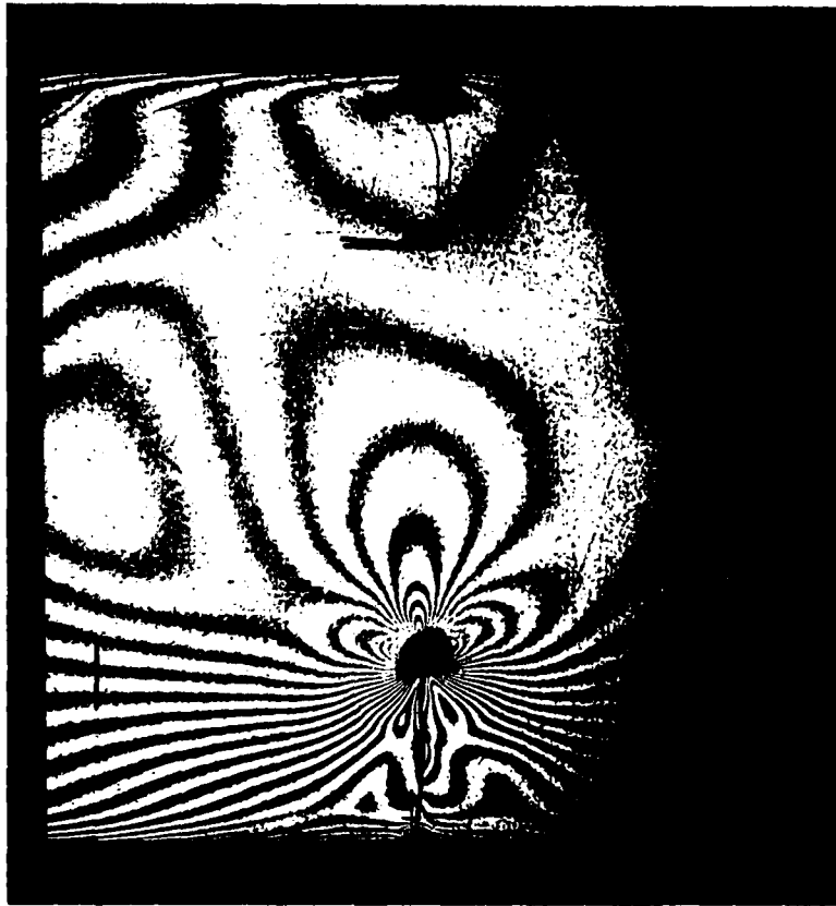
Fig. 16 Photoelastic crack tip fringe pattern
