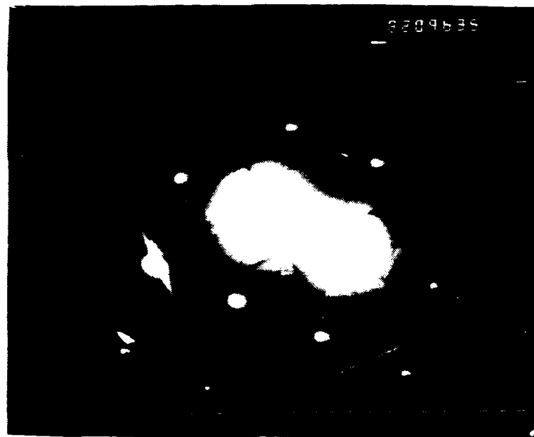
Figure 3.2: Diffraction (TEM) micrograph pair illustrating Kikuchi line shift across a subgrain boundary. Effective camera length was 86.5 cm.
