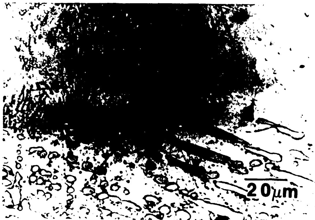
Fig.11. Optical micrograph of a transverse section of a laser surface melted Al-8.0at.%Ni from a region which was not completely melted.
