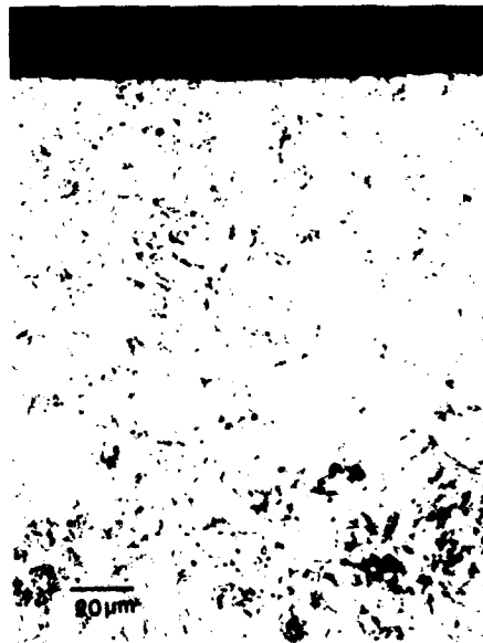
FIG. 10 Optical micrograph through surface after grinding dry at a wheel speed of 18 m/s with graded finishing cuts. There is no detectable change in microstructure.
