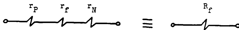
Fig. A.6 Equivalent circuit of a P \pi N diode at forward bias
