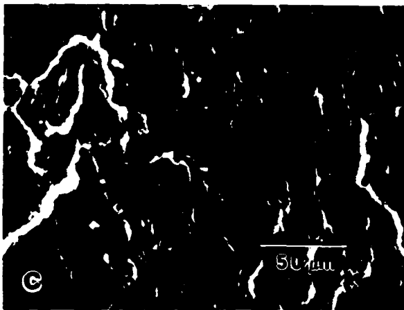
Fig. 24. SEM micrographs of fatigue-tested specimens of extruded Al-4Be ribbon showing a) Fatigue crack in specimen #3 exposed by cutting the backside of the guage section, relative to the crack, and fracturing the remaining portion of the material; b) Crack initiation site in specimen #4, and c) Fatigue striations in region indicated by arrow in "a".
