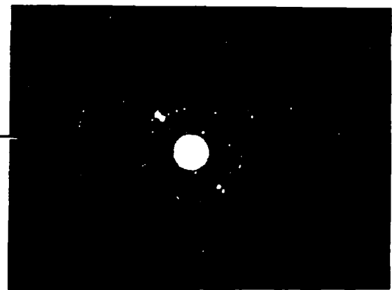
Fig. 45. Bright-field transmission electron micrograph and associated SAD pattern of recrystallized grains within the zone A matrix in dynamically compacted Al-8Fe-2Mo ribbon particulate.
