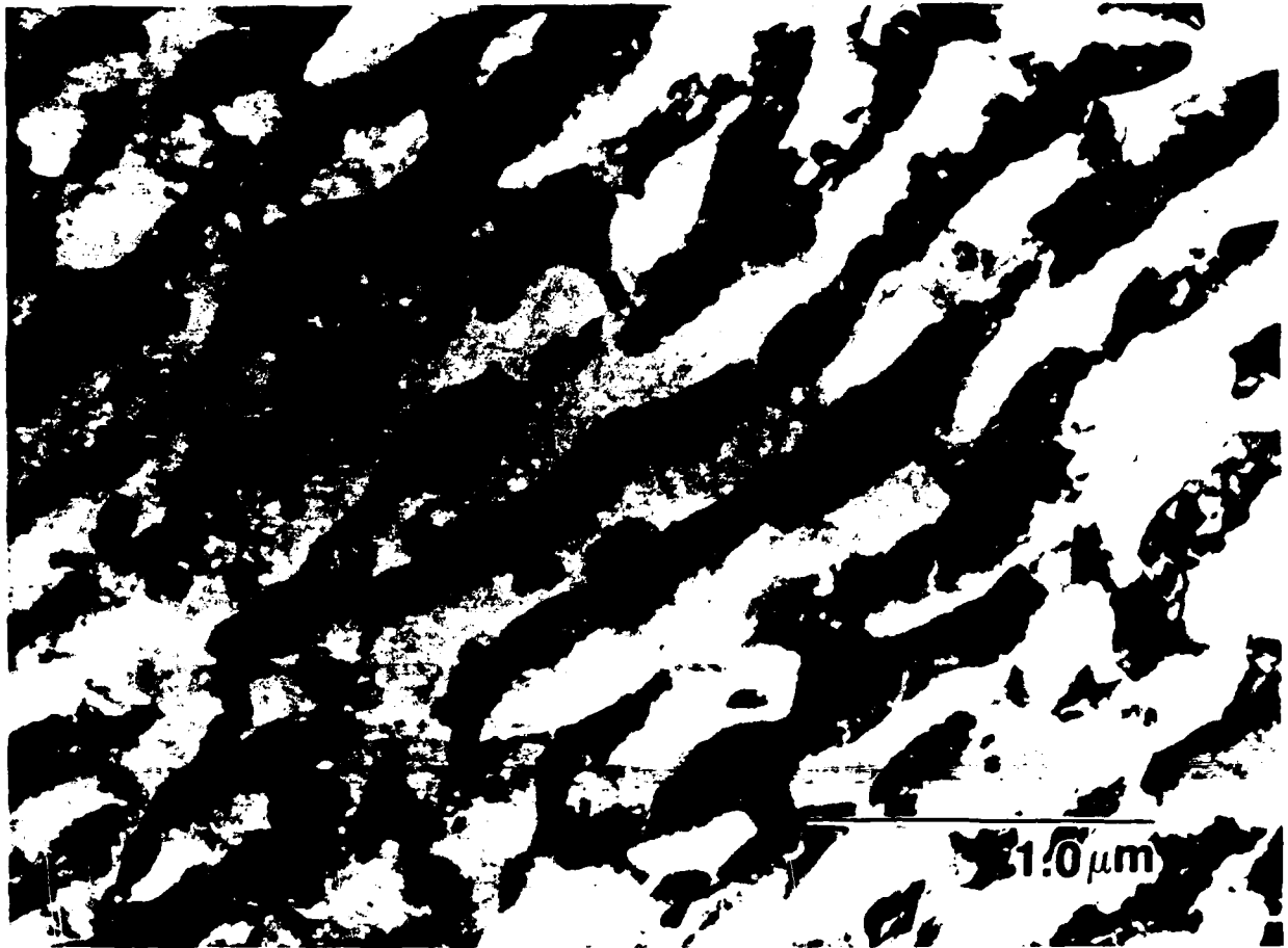
Fig. 60. \alpha lamellae in the \beta grains of as-cast Mg-8Li.
