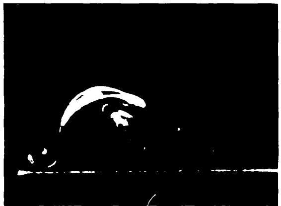
Figure 7. End View. Subharmonic Perturbation Applied at the Leading Edge. Pairing is Enhanced and the Large Vortex is More Organized.
