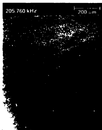
Figure 10 —Grain boundary images of aluminum grains as a function of modulation frequency. The width varies as 1/\sqrt{\omega} .
