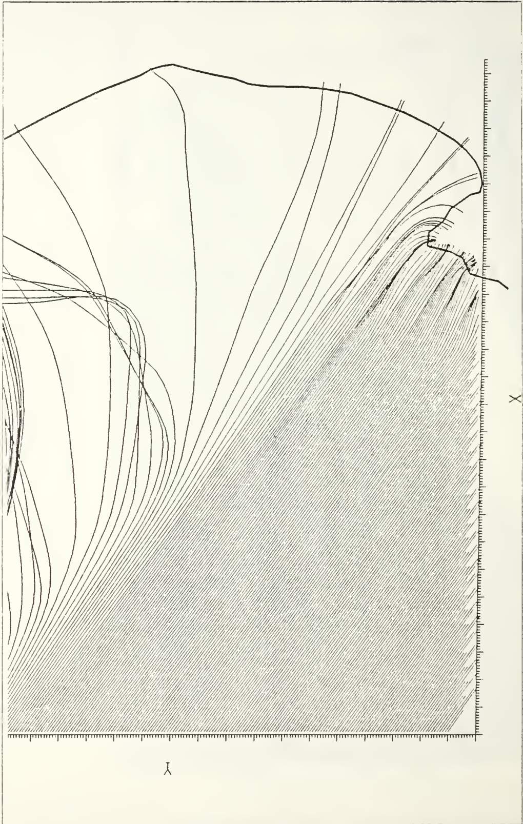
Figure 4.2 Wave Refraction Diagram (Direction: WNW, Period: 25.70 s)
