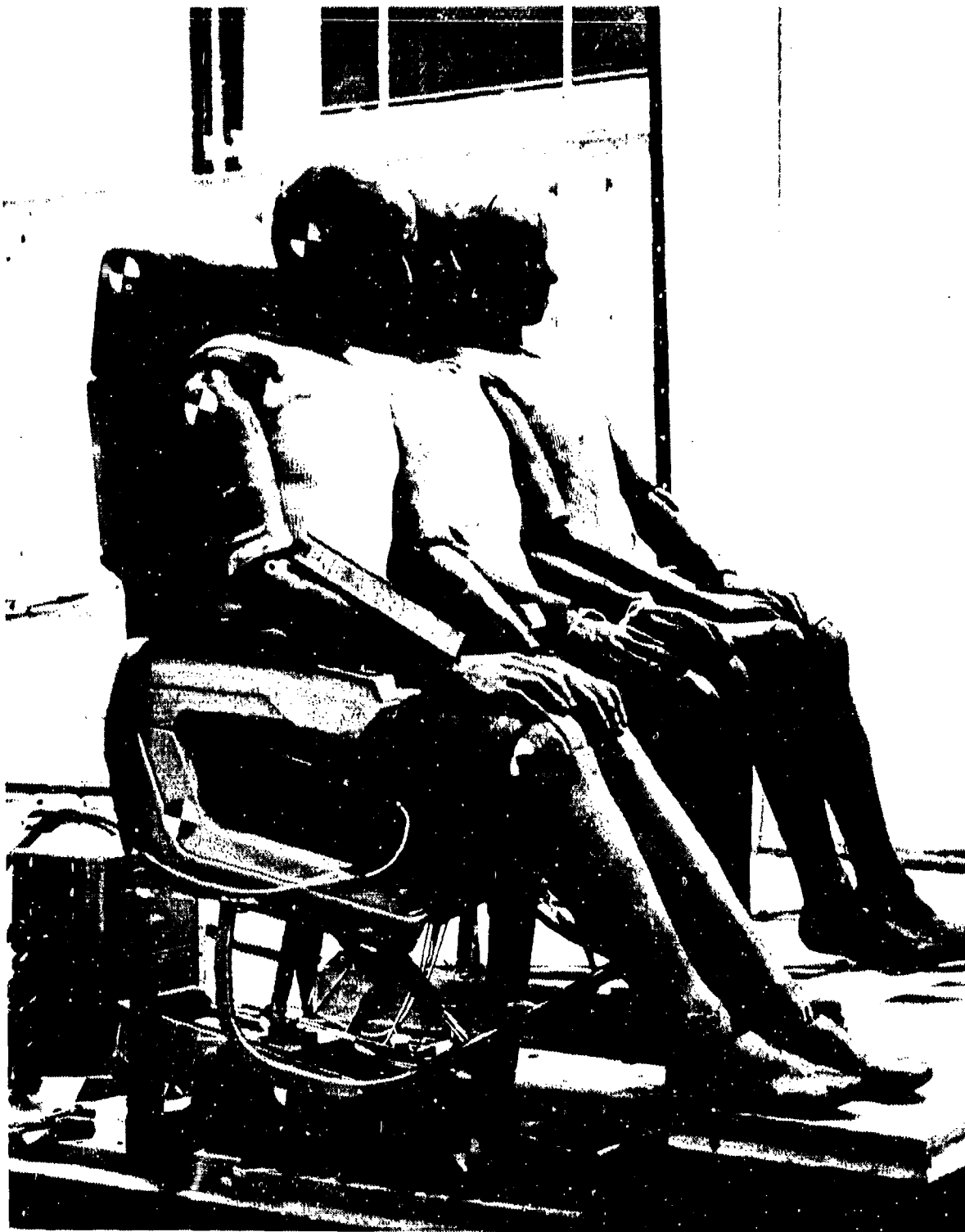
Figure 40. Modified transport aircraft seat and dummies prior to CAMI Test A83-085, aisle-side view (after floor warping).
