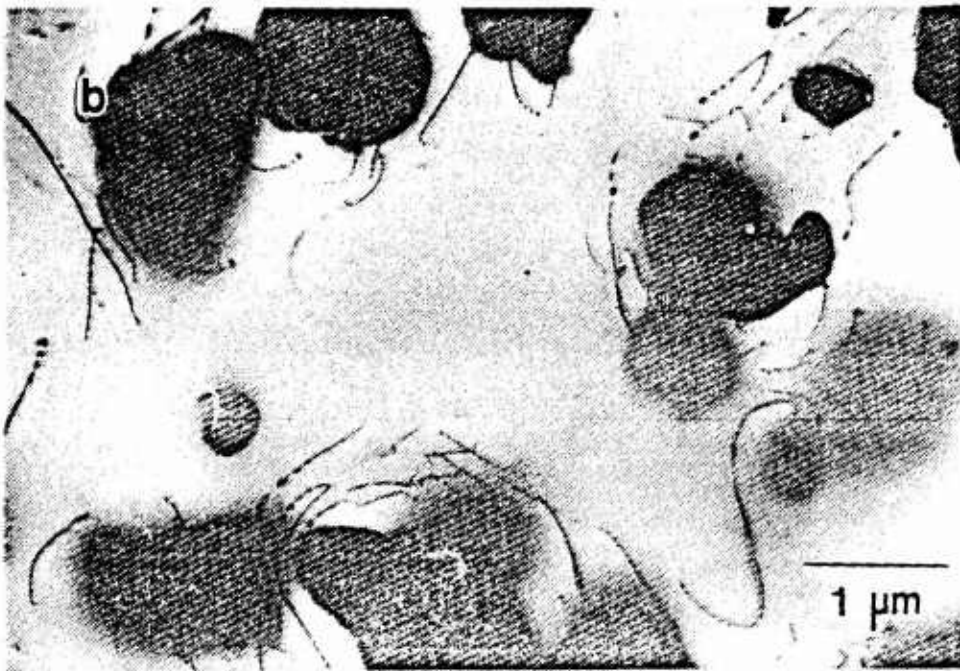
Figure 4.14 TEM micrograph of light reduction Al-10Mg-0.1Zr 633Kscan: (a) Discontinuously recrystallized grains nucleated at \beta (b) \beta in recrystallized grain interiors.
