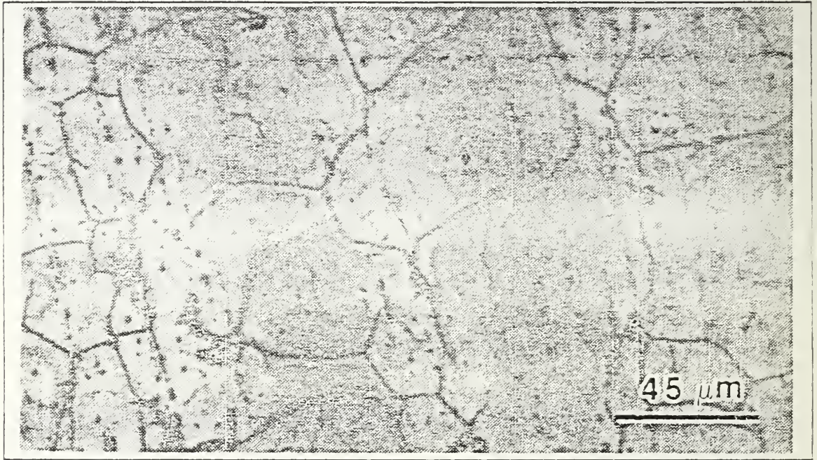
Figure 4.36 Optical Micrograph of 16-Hour Aged INCRAMUTE in the Unstressed Condition Under Normal Light.
