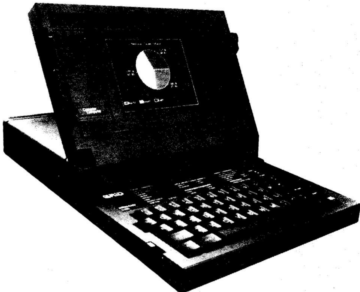
Figure 6. Portable computer with 512K bytes of memory and built in disk drive, fits into a briefcase together with a printer.
