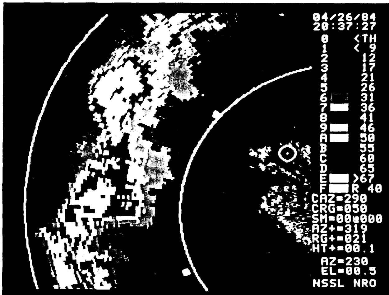
Figure 10. Example of contoured intensity display. The image shows a vertical squall line to the northwest of Norman, Oklahoma, moving to the southeast. The contouring is done to show the intensity of the return and thereby the precipitation intensity. Photo courtesy of the National Severe Storm Laboratory, Norman, OK
