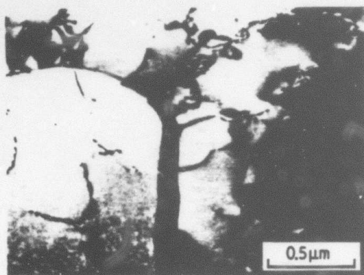
Figure 1 As-spun ribbon of Al-2 wt % Cr alloy. A dislocation substructure is probably associated with slight microsegregation.
