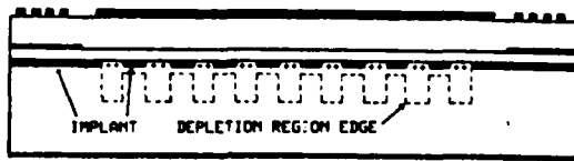
Fig. 7. Schematic of charge storage regions (induced junctions) established beneath the gate of the correlator. Plus signs denote inversion layer charge.
