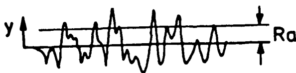
Fig. 25. Average Roughness, R_a
