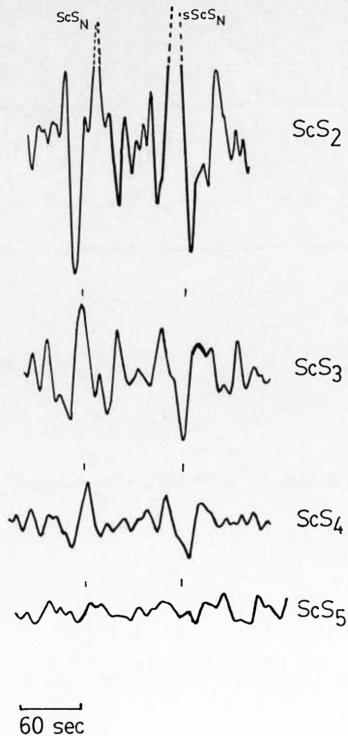
Figure 13 Tracings of multiple ScS phases followed by the corresponding sScS multiples at the WWSSN station SHI for the Hindu-Kush earthquake of 7/03/74.
