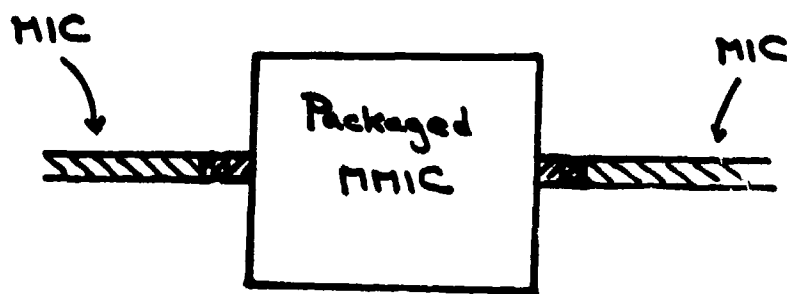
Figure 9 Packaged MMIC to MIC Transition
