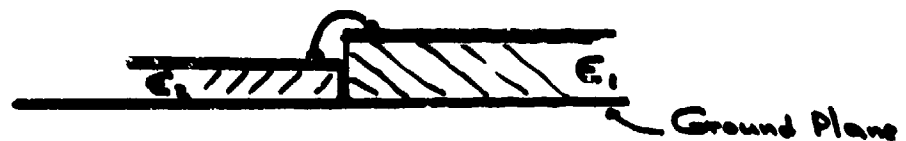
Figure 7 MMIC/MIC Transition, General Case with Different Dielectric Constants and Different Substrate Thicknesses
