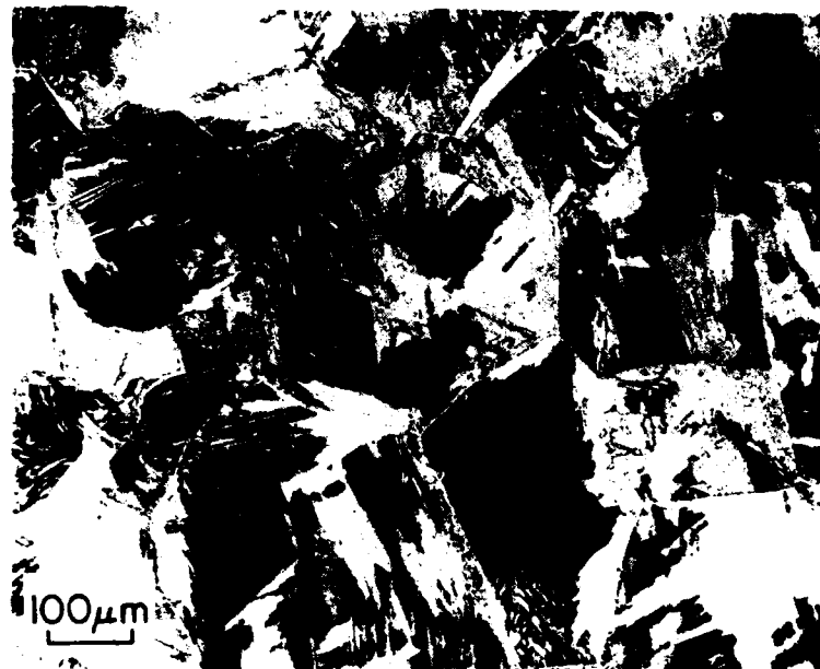
Fig.3.3-1 Light micrograph of Ti-6Al-4V plate material, after beta treatment of 1025°C/10 min/AC.
