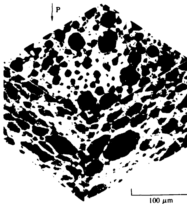
Figure 13. Scanning electron micrographs of aluminum-powder compacts consolidated by uniaxial pressing at 25°C.
