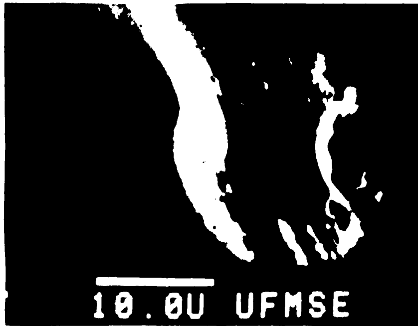
Figure 3 - Clap IA glass heat treated 1 hour at 309C showing the growth of crystals at the droplet-matrix boundary and into the matrix phase.
