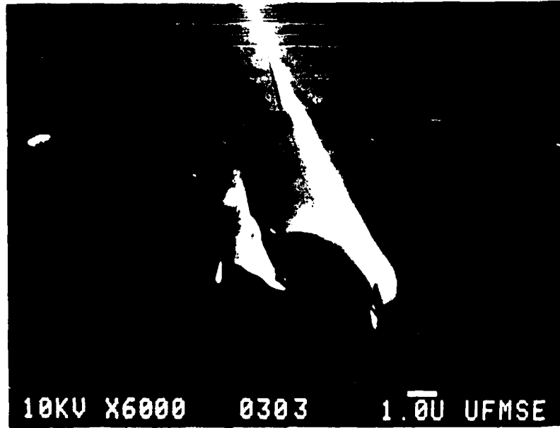
Figure 1a - Amorphous droplet phase in rapidly quenched CLAP IB glass.
