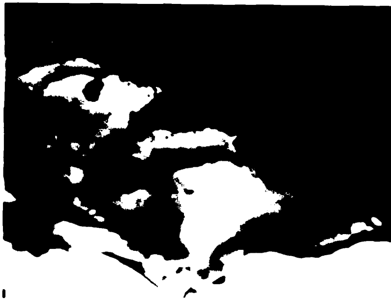
Figure 5 - Dark field TEM picture showing the presence of amorphous spheres.
