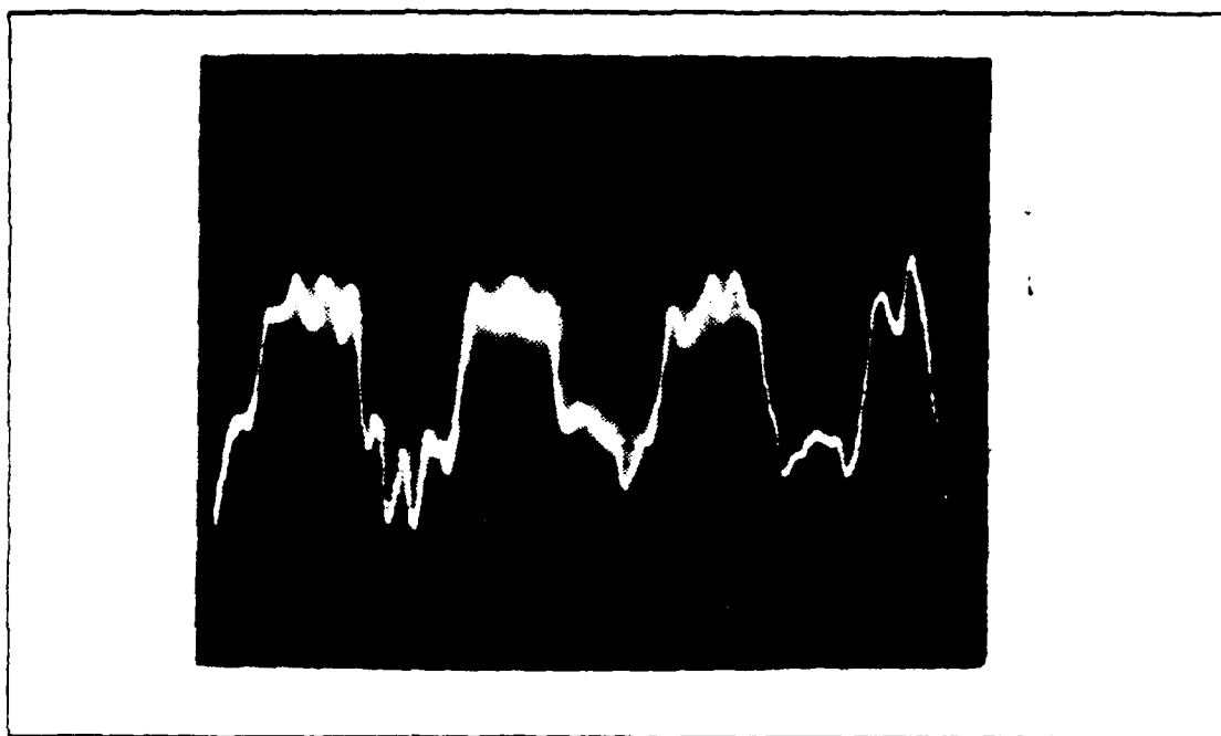
Figure 3.31 Output of the PLL for FSK Modulation Plus Noise (SNR = 4 dB).
